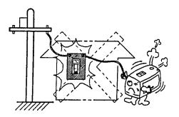
■ Backfeed to a utility system can cause electrocution and/or property damage. Do not connect to any building's electrical system except through an approved device or after building main switch is opened.
